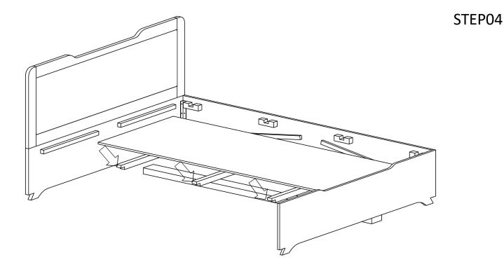
Now Place Part-G(Bottom Panel) into last assembled part as shown in fig.
