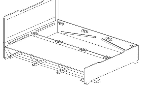
Now place Part-G (Bottom Panel) with last assembled part as shown in Fig.
