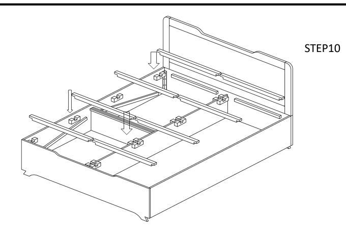
Now fix Part-E (Battens) at upper U-block as shown in Fig.
