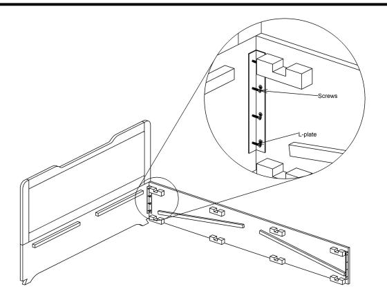
Fix the Part -A(Headboard) and Part-C(Sideboard) on using L-plate with the help of Screw 16mm as shown in fig.
